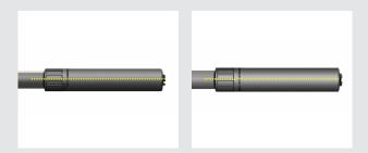
\*NOTE - Barrel threads longer than .630" will utilize the internal shouldering surface, shouldering against the muzzle face, which will create a visible gap externally. While rare, it should be kept in mind.
