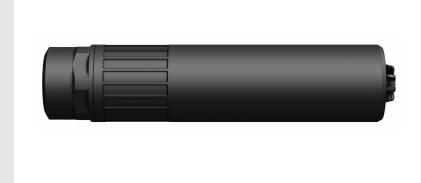
MODEL: CAT/ODB/A1 CALIBER: 7.62×39 (MAX 762NATO) WEIGHT TITANIUM: 9.7 OZ (10.7 OZ MIL) \* WEIGHT INCONEL: 17.9 OZ (21.2 OZ MIL) \* OVERALL LENGTH: 7.20" DIAMETER: 1.60" MIN BARREL LENGTH (TITANIUM): 10" MIN BARREL LENGTH (INCONEL): 8" (5.56NATO) OPTIMIZED VELOCITY: 1100 – 2600FT/S OPTIMIZED PLATFORM: 16" AK47 TECHNOLOGY: SURGE BYPASS RECOMMENDATION: SEMI-AUTO FINISH: DLC MOUNTING: SPOOKY 1 (INCLUDED)
