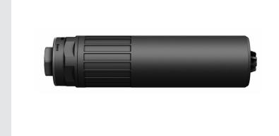
MODEL: CAT/NOAH/A1 CALIBER: 6 ARC WEIGHT TITANIUM: 8.6 OZ (CORE) \* WEIGHT INCONEL: 16.8 OZ (17.5 OZ MIL) \* OVERALL LENGTH: 6.15" DIAMETER: 1.60" MIN BARREL LENGTH (TITANIUM): 10" MIN BARREL LENGTH (INCONEL): 8" (5.56NATO) OPTIMIZED VELOCITY: 1000 – 2800FT/S OPTIMIZED PLATFORM: 14.5" TSF ARC TECHNOLOGY: SURGE BYPASS RECOMMENDATION: SEMI-AUTO 6MM (AND 5.56) FINISH: DLC MOUNTING: 5/8×24 DIRECT THREAD (INCLUDED)
