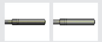
\*NOTE - Barrel threads longer than .630" will utilize the internal shouldering surface, shouldering against the muzzle face, which will create a visible gap externally. While rare, it should be kept in mind.
