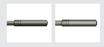
\*NOTE - Barrel threads longer than .630" will utilize the internal shouldering surface, shouldering against the muzzle face, which will create a visible gap externally. While rare, it should be kept in mind.
